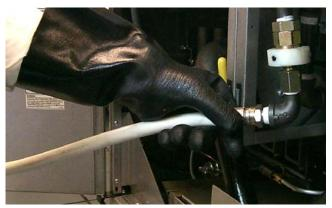
Hose/wand disconnect properly connected to disconnect valve in fryer cabinet (orientation of disconnect may vary according to system).
